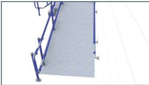
D) CLEARANCE: A ramp must have a minimum clear width of 1m.
