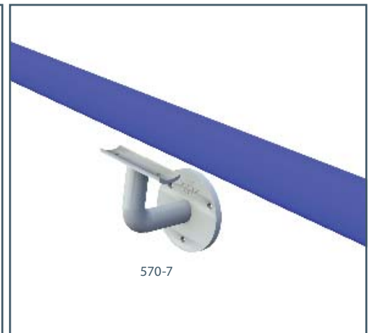
C) WALL MOUNT: The 570-7 is connected to the wall or wood posts using 6mm screws or bolts. The 570-7 is attached to the railing with No. 12 self-drilling screws.
